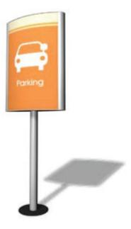
Vista Light's convex post pylon is built of VL style profiles and, a post and a range of bases and end caps. The sign, that can have a permanent or a portable application, can be illuminated with the addition of interior LED lighting. Sign frames and post heights are adjustable.
